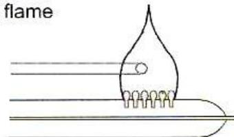
If the flame appearance is not correct (e.g. the flame is yellow or the shape is constantly changing and/or flickering or if the flame is touching metal surfaces inside the burner box – do not use the GAS mode and contact your dealer or authorized Atwood service center.
